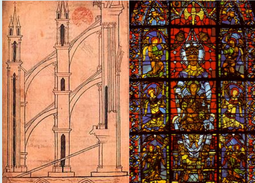
Picture 4: Flying buttresses;
